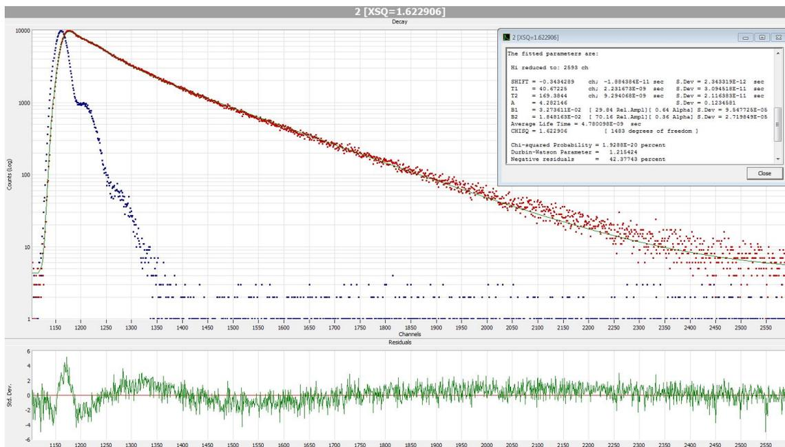
**Figure S40.** Time-resolved fluorescence spectra of CA-Ala with a double exponential fitting (top), output lifetimes (inset), and the fitting residue distribution (bottom)
