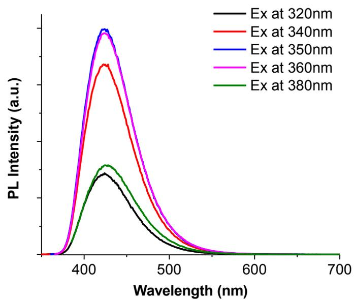
**Figure S3.** Emission spectra of CA-Penicillamine under different excitation wavelengths.
