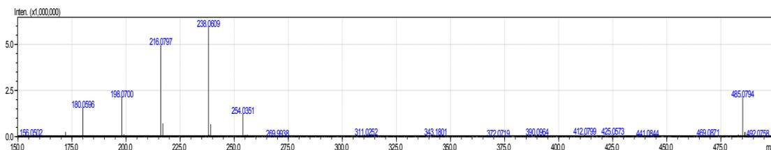
**Figure S25.** ESI-MS spectrum (m/z) of CA-Propylamine. m/z=216: (M+H<sub>2</sub>O+H)<sup>+</sup>;
