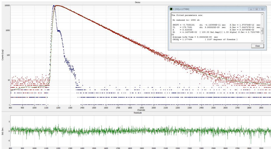
**Figure S38** Time-resolved fluorescence spectra of CA-Cys with a single exponential fitting (top), output lifetimes (inset), and the fitting residue distribution (bottom)
