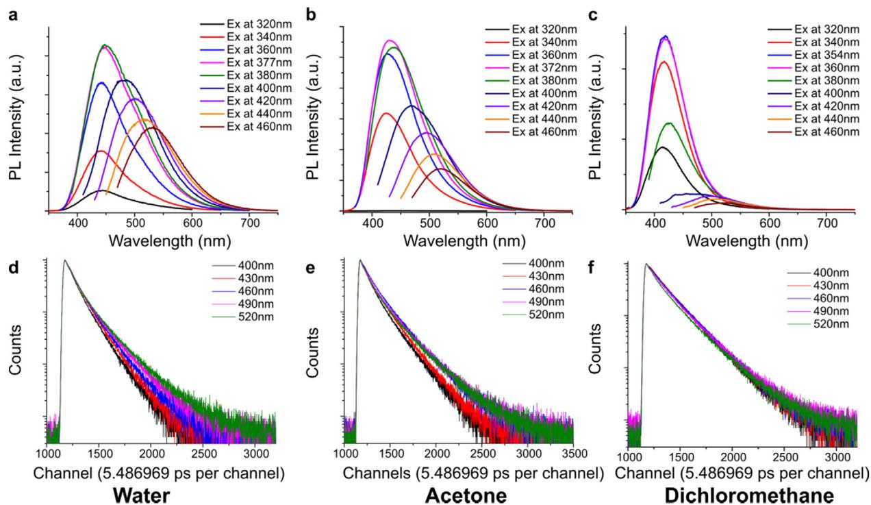
**Fig. 3.** (a–c) Fluorescence emission spectra of CA-Ala at different excitation wavelengths in water, acetone and dichloromethane. (d–f) Fluorescence intensity–time traces of CA-Ala at different emission wavelengths in water, acetone and dichloromethane.
