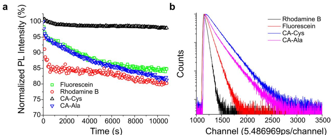
**Fig. 4.** (a) Fluorescence photostabilities of CA-Cys and CA-Ala with 3 h continuous excitation at their respective maximums. Fluorescein and Rhodamine B served as controls. (b) Fluorescence intensity–time traces of CA-Cys, CA-Ala, Fluorescein and Rhodamine B after pulsed excitation at 352 nm.
