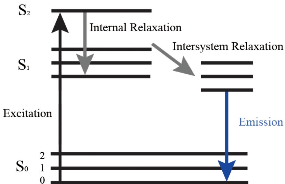
**Figure S5.** A Jablonski diagram of fluorescence excitation and emission processes of a TPA fluorophore.
