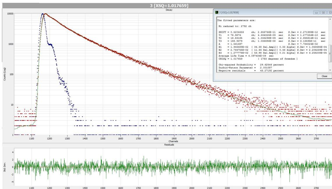
**Figure S41.** Time-resolved fluorescence spectra of CA-Ala with a triple exponential fitting (top), output lifetimes (inset), and the fitting residue distribution (bottom)
