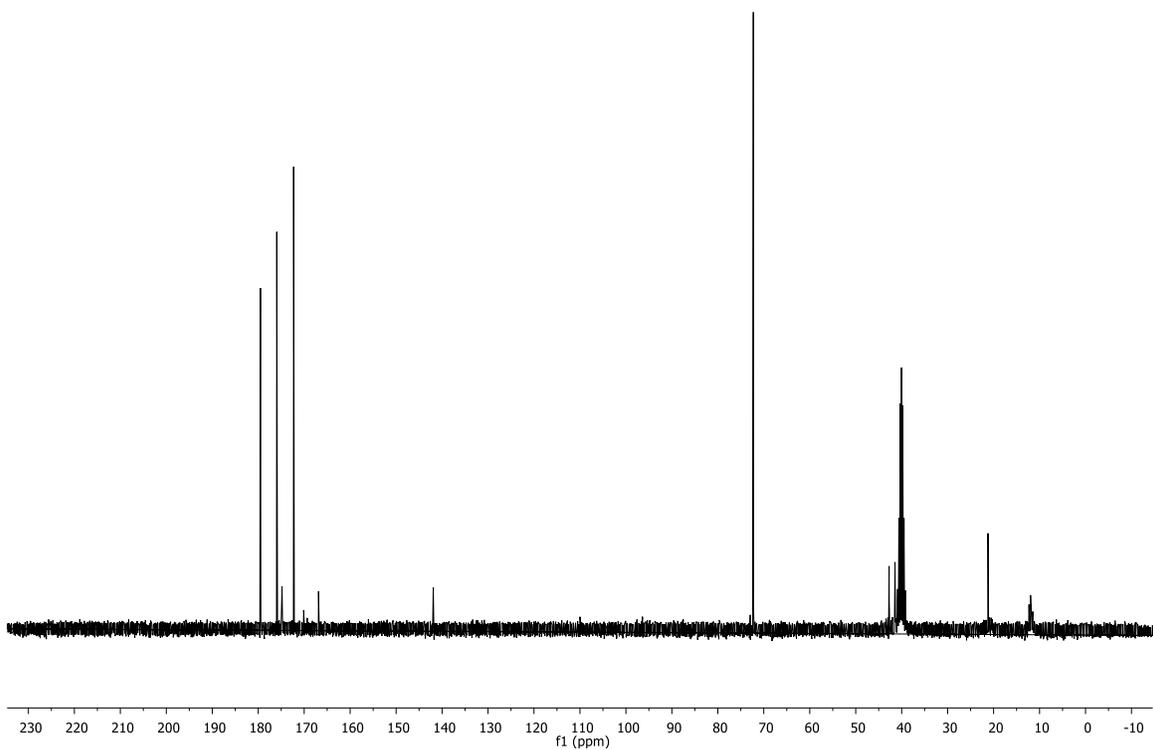
**Figure S27.**  $^{13}\text{C}$  NMR (DMSO- $d_6$ ) spectrum of CA-Propylamine.  $\delta$  179.5, 175.9, 172.3, 166.9, 141.9, 42.74, 40.0, 22.2, 11.9.
