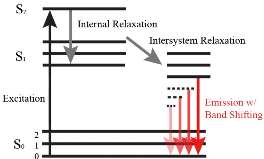
**Figure S12.** A Jablonski diagram of fluorescence excitation and emission processes showing band shifting behaviors of a DPR fluorophore.
