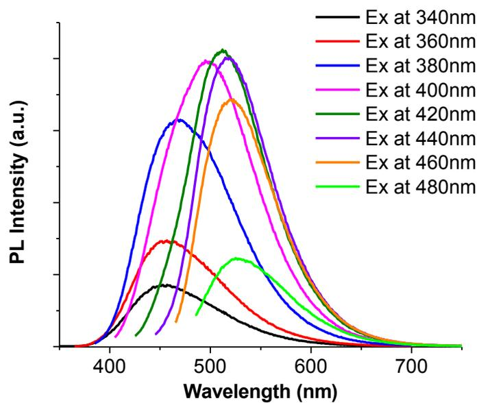
**Figure S10.** Emission spectra of CA-Propylamine at different excitation wavelengths.
