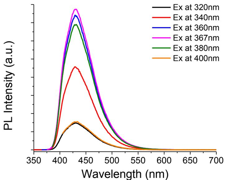
**Figure S6.** Emission spectra of BPLP-TPA under different excitation wavelengths.
