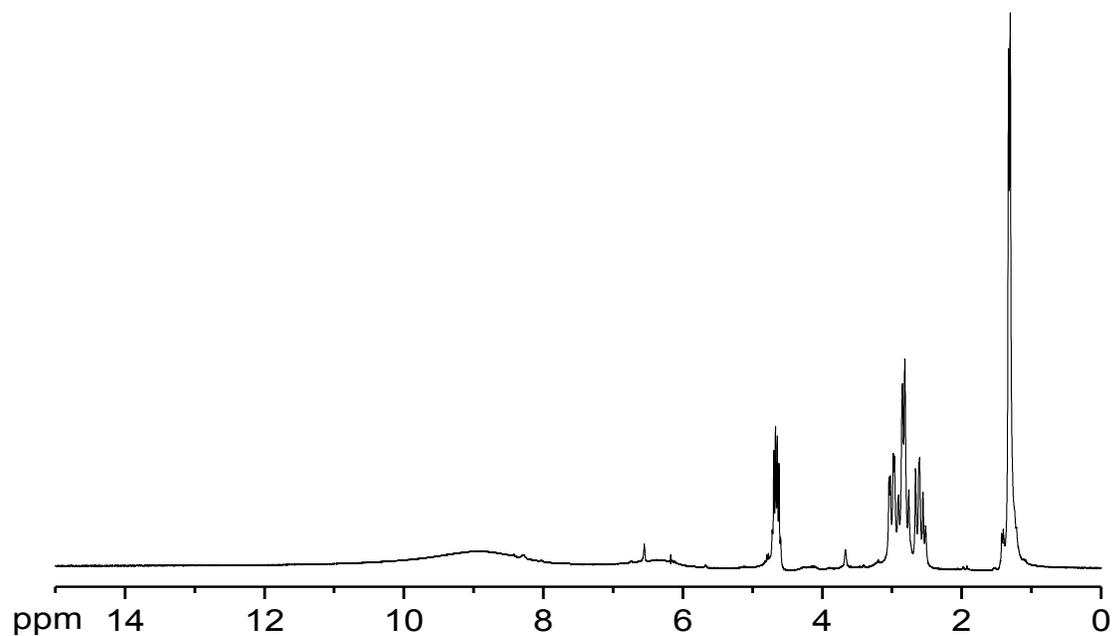
**Figure S30.** <sup>1</sup>H NMR (DMSO-d<sub>6</sub>) spectrum of CA-Ala. δ 4.58-4.78 (m, 1H), 2.50-3.07 (m, 4H), 1.32 (d, 3H).
