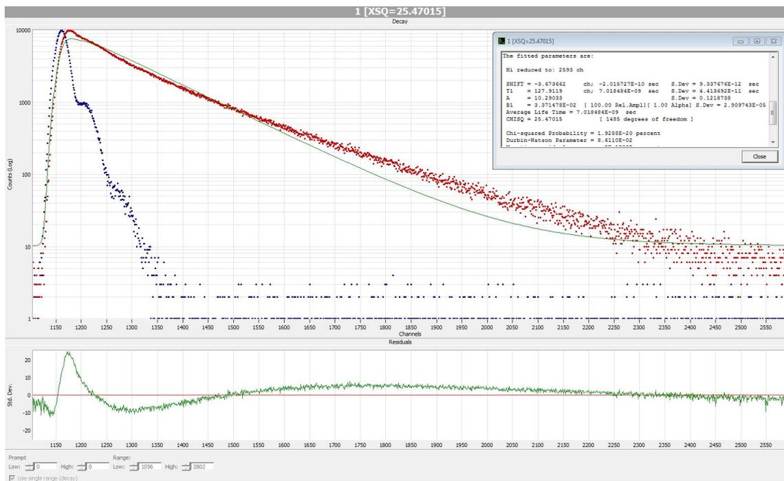
**Figure S39.** Time-resolved fluorescence spectra of CA-Ala with a single exponential fitting (top), output lifetimes (inset), and the fitting residue distribution (bottom)
