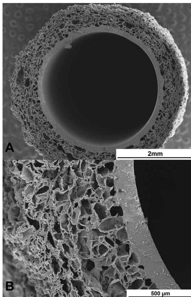
**FIGURE 1.** Cross-section of CUPE biphasic scaffold with non porous inner phase and porous outer phase (A). High magnification image showing pore structure of porous phase and seamless integration of the two phases (B). Magnification: (A) 20 $\times$  and (B) 80 $\times$ .
