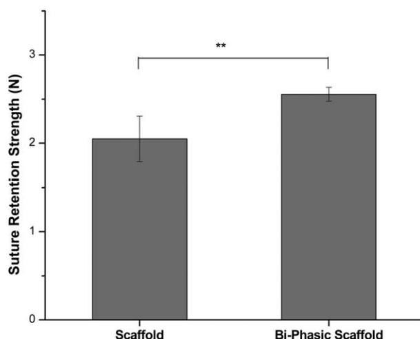
**FIGURE 4.** Suture retention strength of biphasic CUPE scaffolds. Salt leached CUPE scaffold served as control. \*\* Corresponds to  $p < 0.01$ .  $N = 5$  for both biphasic scaffold and control.
