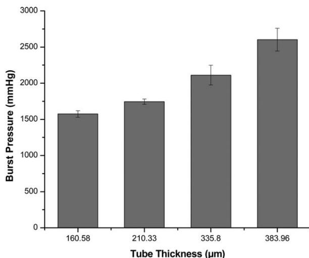
**FIGURE 3.** Effect of non porous tubular wall thickness on measured burst pressure of CUPE tubes (80°C, 4 days) ( $N = 4-8$ ). Burst pressure of tubes increased with increasing wall thickness.
