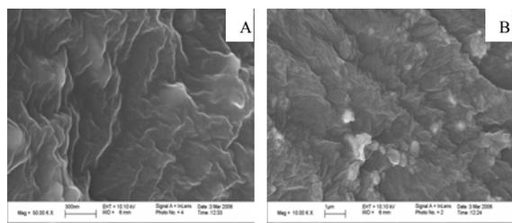
Figure 2. SEM pictures of POC-PEGDM (nano-POC) films. A) surface morphology, scale bar=300 nm; B) cross-section. scale bar=1 μm.
