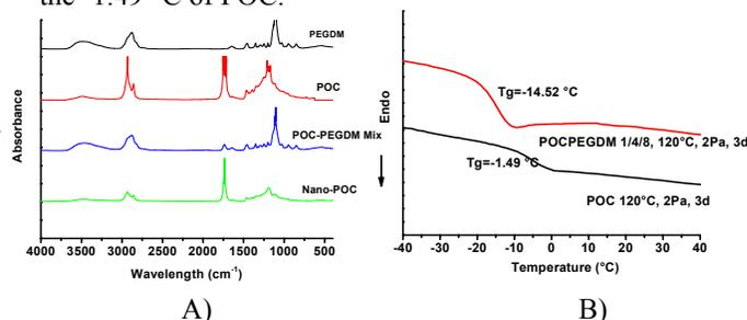
Figure 1: A) FTIR spectrum of PEGDM, POC, POC-PEGDM mix, and nano-POC after PEGDM leaching; B) DSC thermograms of POC and nano-POC.
