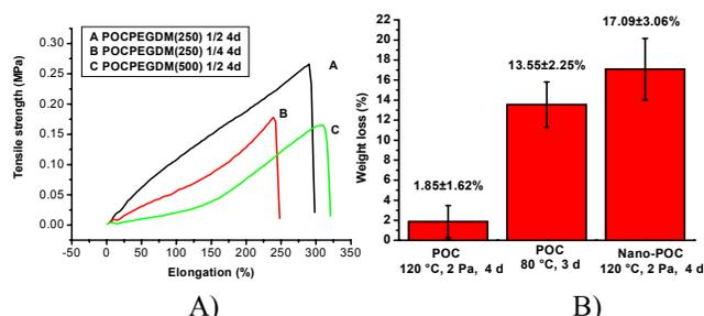
Figure 3: A) Stress-strain curves of POC-PEGDM films; B) Degradation profiles of POC and POC/PEGDM 1/2/8 scaffolds over a period of 6 weeks in PBS at 37 °C.
