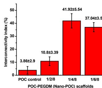
Figure 5: Interconnectivity index of nano-POC scaffolds with POC/PEGDM250/salt ratio of 1/2/8, 1/4/8, and 1/6/8 and POC control scaffolds.
