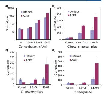
**Figure 3.** Comparison of the sensor performance based on diffusion and ACEF enhancement (square wave potential of 5 V<sub>pp</sub> and 200 kHz) with an incubation time of 8 min for detecting (a) different concentrations of *E. coli* clinical isolates in culture media, (b) *E. coli* in clinical samples urine 105.2 and urine 74 with  $4 \times 10^4$  cfu/mL and  $4 \times 10^6$  cfu/mL *E. coli*, respectively, (c) *S. saprophyticus* clinical isolates, and (d) *P. aeruginosa* clinical isolates.
