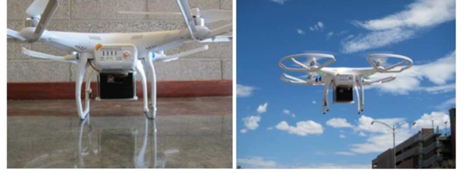
Fig. 3. Flying test. The system is attached to the bottom of quadcopter. Maximum flight time is approximately 20 minutes.
